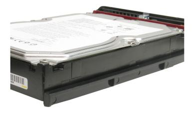
**Step 4** Line up the guides with the case, and slide the hard drive back in. The enclosure should slide shut.
